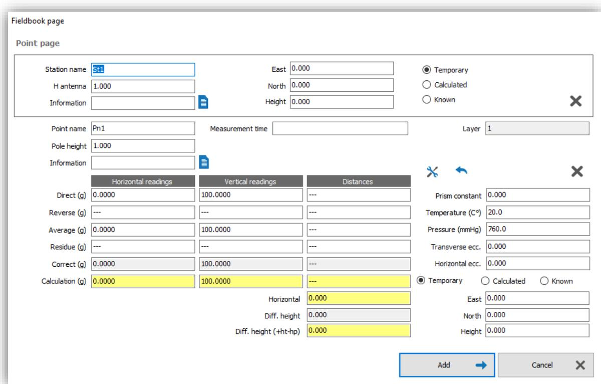
The screenshot shows the 'Fieldbook page' with a 'Point page' section. It contains several input fields for station and point information, a table of calculation results, and a section for measurement parameters.
